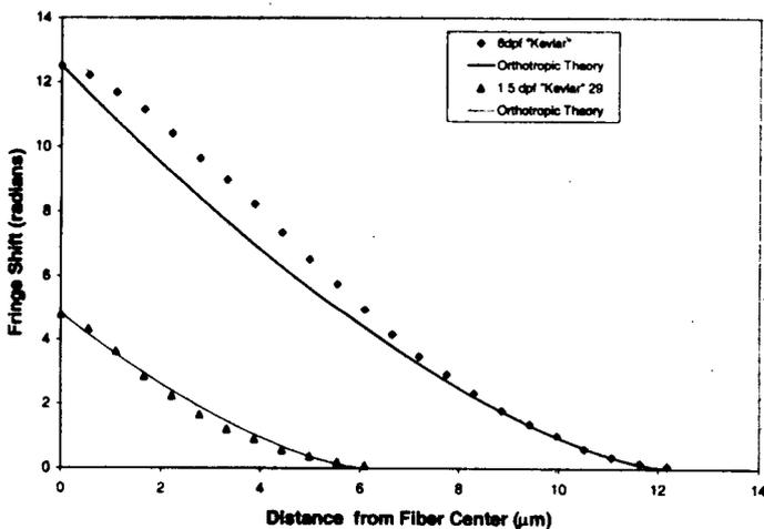
FIGURE 3. Interference fringe profile for Kevlar fibers.
