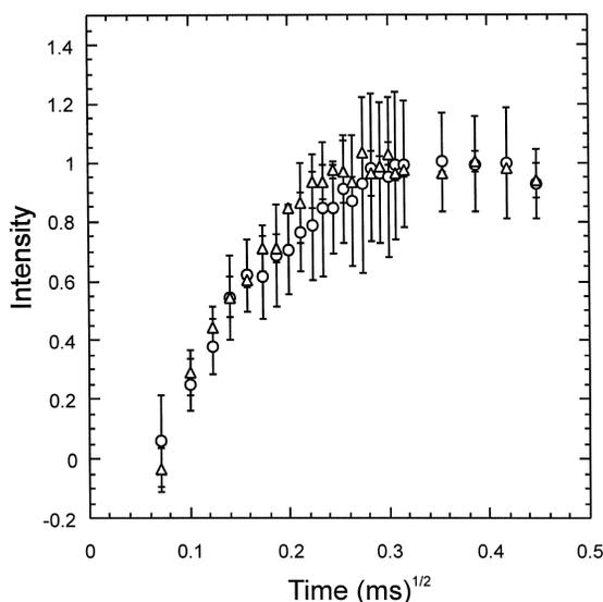
Fig. 5. A plot of magnetization recovery for the poly(styrene-*b*-isoprene-*b*-styrene) triblock copolymer following the dipolar filter. The data are shown for the ( $\Delta$ ) clear and ( $\circ$ ) honeycomb film.
