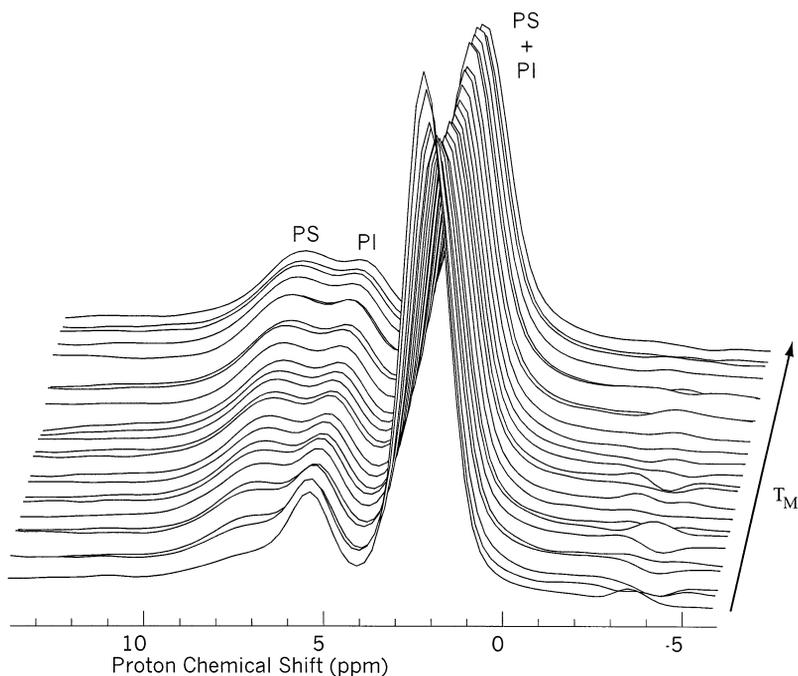
Fig. 4. The solid-state proton NMR spectra of the poly(styrene-*b*-isoprene-*b*-styrene) triblock copolymer as a function of the delay time between the saturation pulse train and observation. The delay time  $\tau_m$  varies between 50  $\mu$ s and 50 ms.
